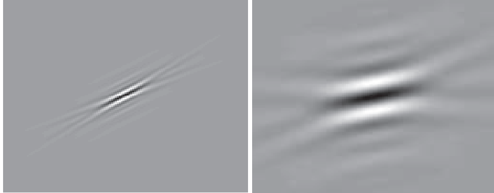
Figure 4: Two example curvelets. The left panel represents a curvelet at a finer spatial scale. The right panel shows a curvelet at a coarser spatial scale.
