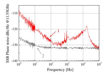
Fig. 3. Relative Residual phase noise of the optical-to-microwave division process (Curve 1). Curve 2: readout noise floor of the carrier suppression noise measurement system
