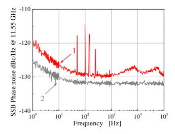
Fig. 7. Single-Side-Band (SSB) phase noise power spectral density of microwave signal at 11.55GHz measured by the Carrier Suppression Noise Measurement System (CSNMS). Curve 1: voltage control phase shifter and pump-current-based power lock scheme applied for phase noise reduction. Curve 2: readout noise floor of the CSNMS.
