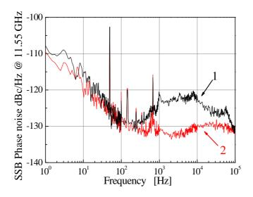
Fig. 6. Curve 1: Single-side-band (SSB) phase noise power spectral density measured without phase noise correction. Curve 2: voltage-controlled phase shifter into low bandwidth fiber-based optical frequency comb for residual feed-forward phase noise correction.
