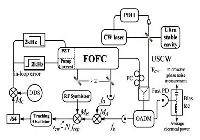
Figure 1 Experimental setup. FOFC: fiber-based optical frequency comb; USCW: ultra-stable continuouswave laser; PDH: Pound-Drever-Hall; PC: polarization controller; OADM: optical add/drop module; DDS: direct digital synthesizer.
