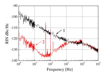
Fig. 4. Curve 1: Relative intensity noise (RIN) of the femtosecond comb. Curve 2: RIN with acousto-opticmodulator-based power lock
