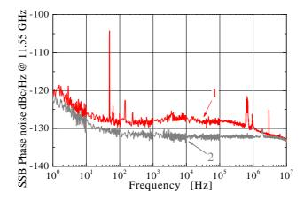
Fig. 10. Curve 1: pump-current-based power lock for near-carrier excess phase noise reduction and two voltage control phase shifters for phase correction. Curve 2, readout noise floor of the carrier suppression noise measurement system.
