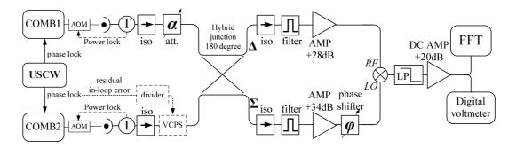
Figure 2. Carrier-suppression noise measurement system. T: bias- tee; Iso: isolator;  $\alpha$ : attenuator; filter: band-pass filter at 11.55GHz; AMP: low-noise amplifier;  $\phi$ : phase shifter; LP: 50MHz low-pass filter; DC AMP: low noise DC amplifier; FFT: Fast Fourier Transform analyzer; VCPS (in dash line): voltage control phase shifter; Divider (in dash line): voltage divider.
