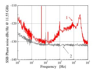
Fig. 5. Curve 1: Residual phase noise of the optical-to-microwave division process with the acousto-opticmodulator-based power lock for near-carrier excess phase noise reduction. Curve 2: readout noise floor of the carrier suppression noise measurement system.
