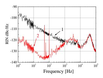
Fig. 8. Relative intensity noise (RIN) measurement based on the out-of-loop fast photodiode. Curve 1: RIN with frequency lock. Curve 2: RIN with frequency lock and pump-current- based power lock.
