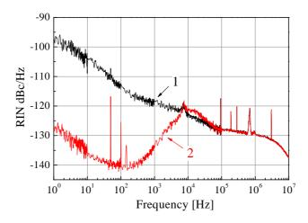
Fig. 9. Curve 1: Relative Intensity Noise (RIN) without power stabilization. Curve 2: RIN with pump-current-based power lock.
