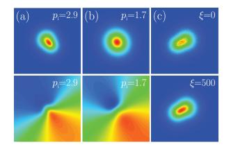
FIG. 4: (Color online) Field modulus (top) and phase (bottom) distributions in asymmetric dissipative solitons for  $p_i =$ 2.9 (a) and  $p_i =$  1.7 (b) at  $\alpha =$  1.9, d = 1.5. (c) Stable propagation of a perturbed asymmetric soliton at  $p_i =$  2.0,  $\alpha =$  1.2, d = 1.5. Initial and final field modulus distributions are shown.
