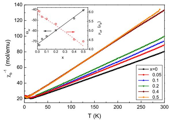
FIG. 2. (Color online) Inverse magnetic susceptibility of  $\text{Mn}_{1-x}\text{Zn}_x\text{WO}_4$ . The inset shows the  $x$ -dependence of the estimated effective magnetic moment  $\mu_{eff}$  and the Curie-Weiss temperature  $\theta_W$ . The dashed line is the expected  $\mu_{eff}$  for an Mn spin of  $S=5/2$ . The black (solid) line is a linear fit to the data of  $\theta_W$ .
