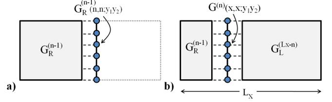
FIG. 3. (Color online) Schematic depiction of recursive Green's function method (eq. 8,9). (a) Green's function for the end of an  $L_x$ -layer sample  $G^{(L_x)}$  is calculated recursively from  $G^{(n-1)} \rightarrow G^{(n)}$  by adding one transverse layer at a time. (b) Green's function for any layer can then be recovered from solving (9) for the desired location, using the intermediate results for  $G^{(L_x-x)}$  and  $G^{(x-1)}$  from the top procedure.
