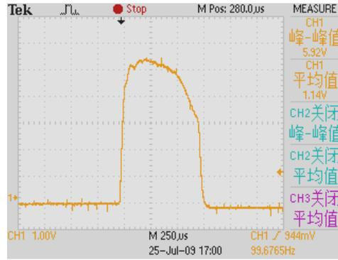
Fig 9 The accelerated beam by SFRFQ was recorded by a faraday cup with a 10koms sample resistor
