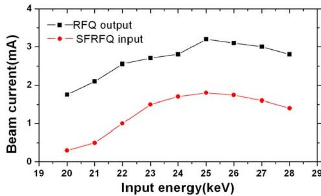
Fig 7. The input energy of RFQ vs output beam current of RFQ and input of SFRFQ
