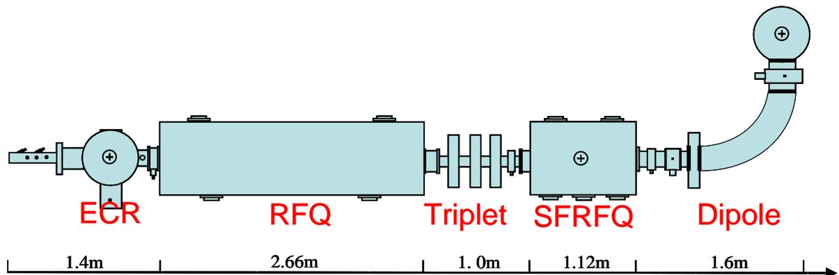
Fig 1. Layout of RFQ and SFRFQ combined accelerator system
