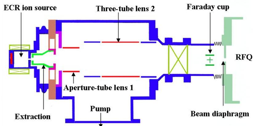
Fig 2 ECR ion source and Low energy beam transmission (LEBT)
