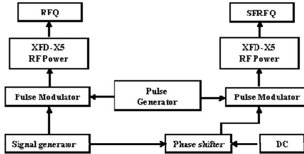
Fig 3. The schematic of rf power feeding
