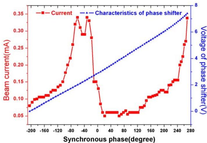
Fig 8 Synchronous phase vs beam current of SFRFQ, and the characteristics of phase shifter (the beam current is a function of synchronous phase and it can be repeated after 360 degree)
