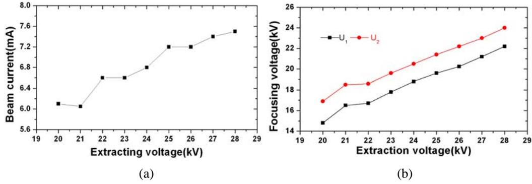
Fig 4 Extracting voltage against beam current of Ion source (a) and focusing voltage (b)
