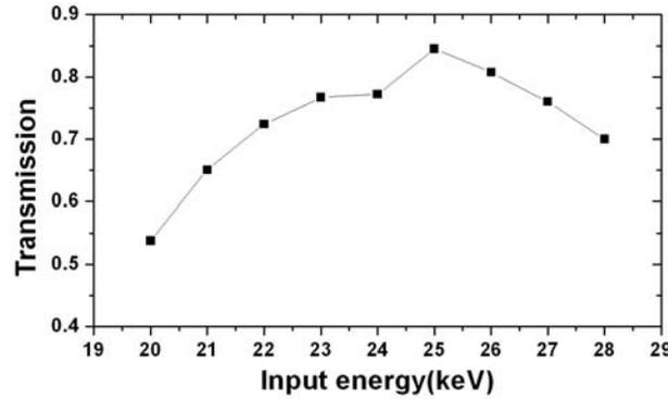
Fig 5. Input energy vs. RFQ transmission
