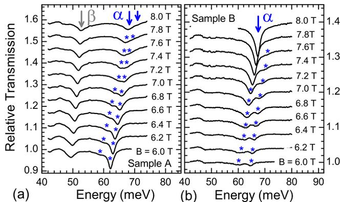
FIG. 4: Detail of magneto-transmission spectra for samples A and B in parts (a) and (b), respectively, which show two components of the  $\alpha$  line at magnetic fields close to the crossing field  $B_c$ .
