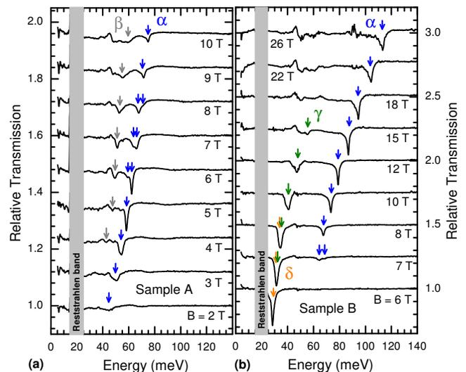
FIG. 2: Transmission spectra of both investigated samples in a relevant range of magnetic fields. The notation of the observed lines follows Ref. 14 and is in agreement with the transitions' assignment used in Fig. 1. Samples are completely opaque in the range of the HgTe/HgCdTe reststrahlen band (14-25 meV).
