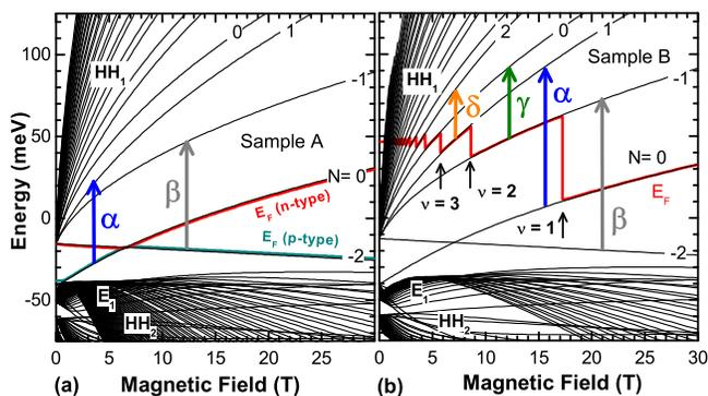
FIG. 1: Calculated dispersion of Landau levels for both studied samples. The expected dominant absorption transitions are denoted by arrows and Greek letters. Whereas the  $\alpha$  and  $\beta$  lines should be observable in both samples, the  $\gamma$  and  $\delta$  transitions are directly related to the presence of 2DEG in the sample B. The Fermi level is shown in both cases by a solid line. Two lines for  $E_F$  are plotted for the sample A, as the type of the residual doping is not known.
