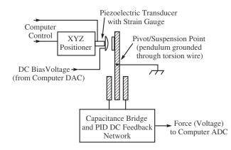
FIG. 1: The top-view schematic of the torsion-pendulum experimental apparatus.
