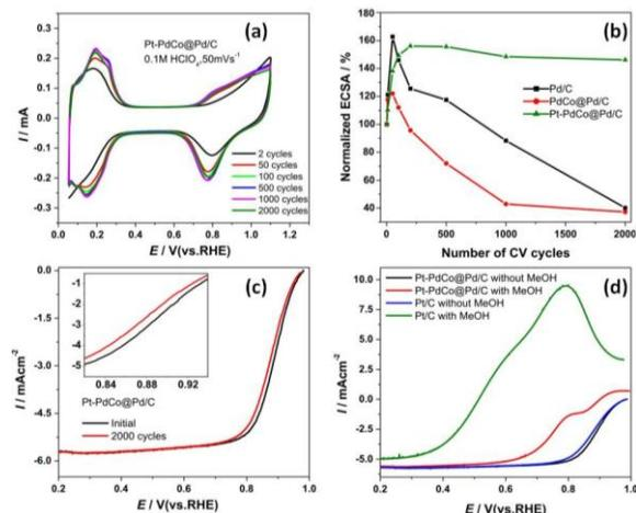
**Figure 3.** (a) CVs of the Pt decorated PdCo@Pd/C after different number of potential cycles. (b) loss of ECSA of different catalysts with number of CV cycles in  $N_2$ -purged 0.1 M  $HClO_4$  solution. (c) ORR polarization curves of Pt decorated PdCo@Pd/C catalyst before and after cycling. (d) Polarization curves of Pt-PdCo@Pd/C and Pt/C in  $O_2$ -saturated 0.1 M  $HClO_4$  in the presence of 1 M MeOH. rotation rate: 1600 rpm, sweep rate:  $5\text{ mV s}^{-1}$ .
