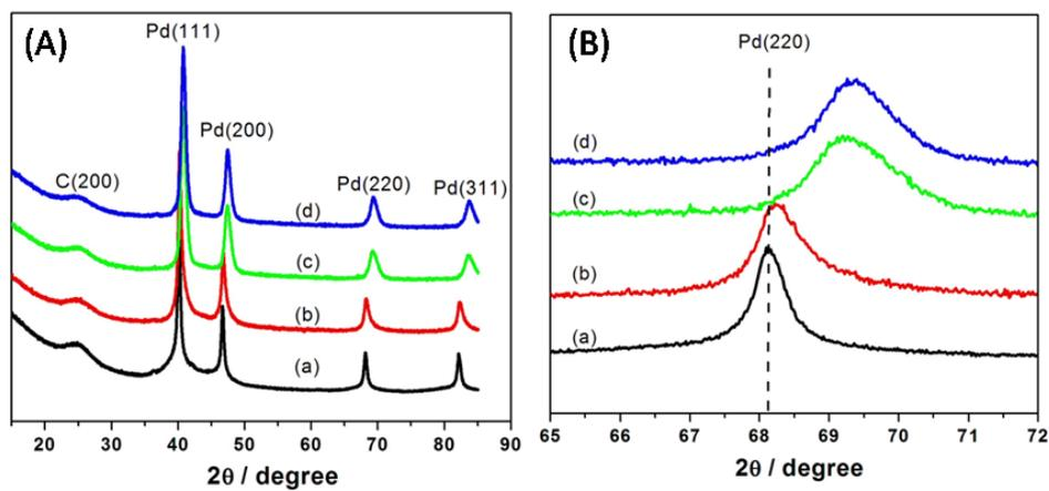
**Figure S4.** (A) XRD patterns of Pd/C(a), PdCo/C(b), PdCo@Pd/C(c) and Pt-PdCo@Pd/C(d); (B) Expanded view of the Pd(220) diffraction peaks of different samples.
