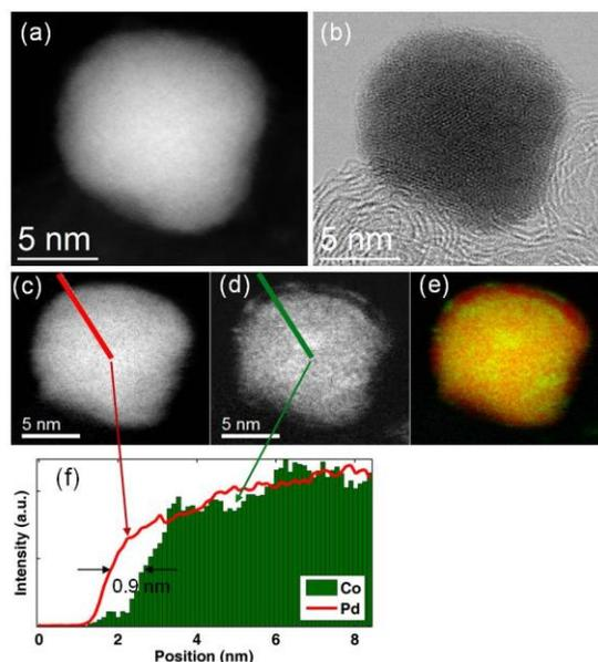
**Figure 1.** Annular dark-field (ADF) (a) and bright-field (BF) (b) STEM image of core-shell PdCo@Pd nanoparticle, EELS mapping of Pd (c), Co (d) and overlay of Pd (red) vs Co (green) (e), EELS line profiles of Pd and Co showing the Pd shell (f).
