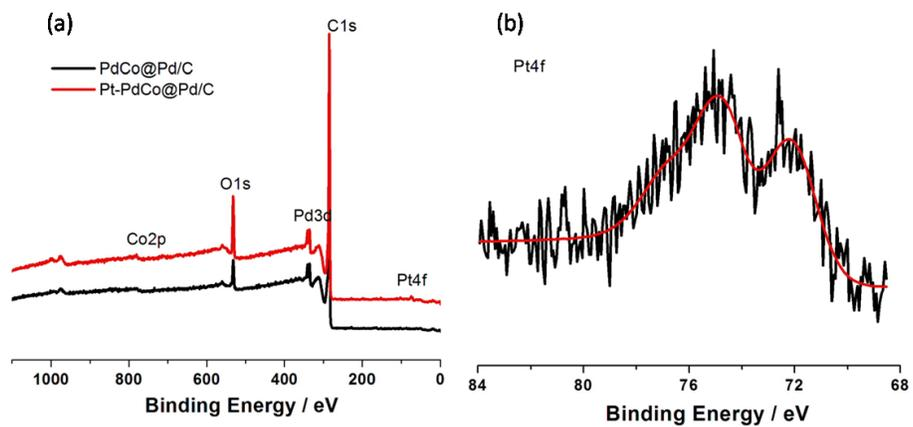
**Figure S5.** Wide-range XPS of PdCo@Pd/C and Pt-PdCo@Pd/C samples (a) and Pt 4f fine spectra (b).
