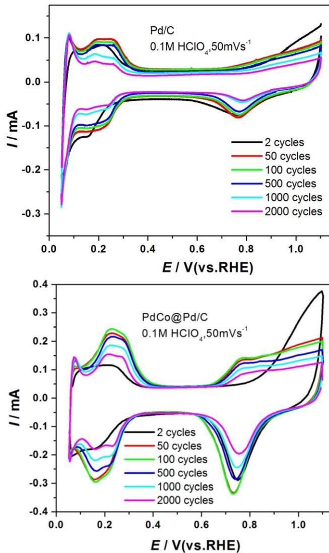
**Figure S6.** Curves of the Pd/C and PdCo@Pd/C catalyst changed with different scanning cycles.
