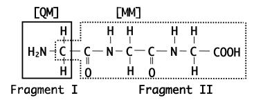
FIG. 3: Fragmentation of glycine trimer used here[9]. QM means the fragment treated by quantum mechanical dynamics while MM the part handled as an environment for QM giving classical electrostatic field.
