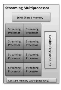
FIG. 2: Schematic picture of a Streaming Multiprocessor (SM).
