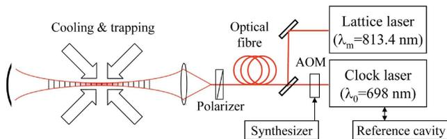
FIG. 5 (Color online) Schematic diagram of the experimental setup for Sr spectroscopy used in an early experiment (Takamoto and Katori, 2003). Ultracold  $^{87}\text{Sr}$  atoms are loaded into a 1D optical lattice produced by the standing wave of a Ti-sapphire laser tuned to the magic wavelength. The atoms interact with the clock laser propagating along this axis and the Lamb-Dicke condition is satisfied. AOM, acousto-optic modulator.
