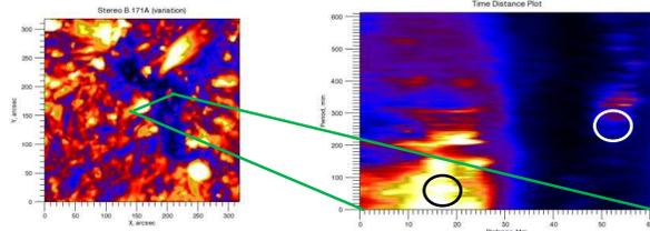
**Fig. 6** Time shifts and distance measurements. Left: Variation map of the observational data; green line shows the profile direction. Right: time-distance plot through the line connecting eruption location and oscillating loop. Black circle shows eruptive event location, white circle shows the start of the loop oscillation.
