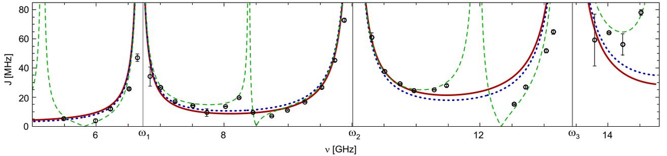
FIG. 4: Exchange coupling  $J$  versus qubit frequency in sample B. The vertical lines indicate the frequency of the coplanar waveguide modes  $\omega_j$ . Experimental data (dots) confirm the expected increase of  $J$  with increasing frequency. The solid red (dotted blue) line indicates the calculated  $J$  including  $N = 6$  ( $N = 7$ ) resonator modes. The dashed green line is a fit to a model with additional resonances.
