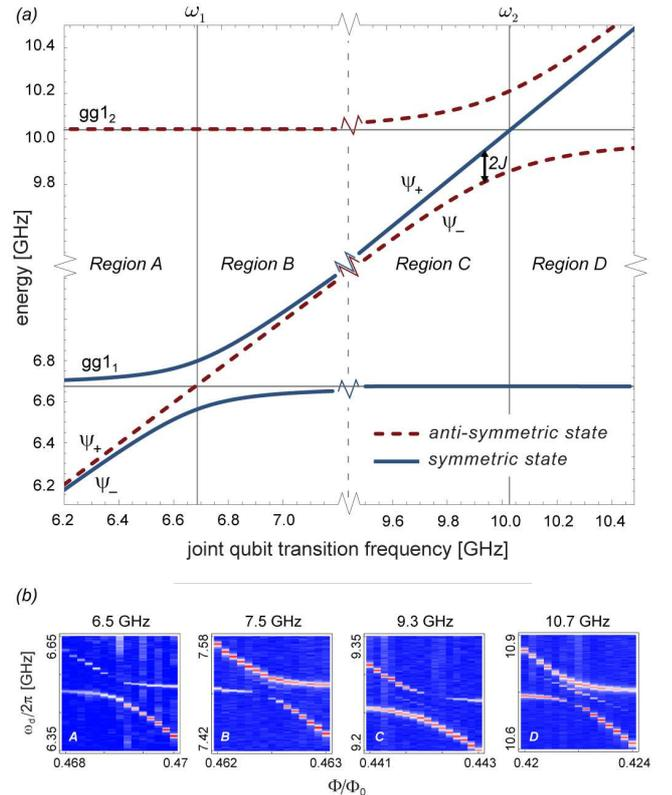
FIG. 5: (a) Energy levels of the qubits-resonator system when the qubits are degenerate and their transition frequencies are simultaneously swept across the resonator modes. The parameters are those of sample B (Table I). (b) Spectroscopic measurements of the anti-crossing in the regions labeled A, B, C and D in (a).
