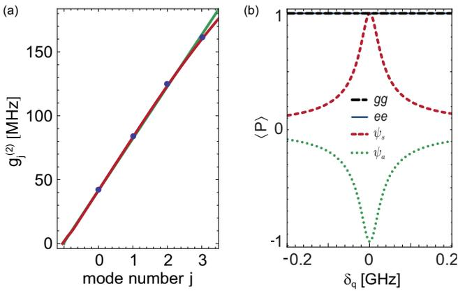
FIG. 6: (a) Coupling strength  $g_j^{(2)}$  of qubit 2 to the  $j$ -th harmonic mode in sample B. (b) Expectation value of the permutation operator  $P$  for the eigenstates of the Jaynes-Cummings Hamiltonian as a function of qubit-qubit detuning  $\delta_q$ .
