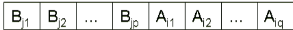
FIG. 2: Encoding schema of a chromosome for a bipartite network (p, q) . B_{j_k} (for k \leq p ) is the allele at the locus representing node A_k , which stands for a neighbor node of A_k in the network. Similarly, A_{i_k} (for k \leq q ) is the allele at the locus representing node B_k .
