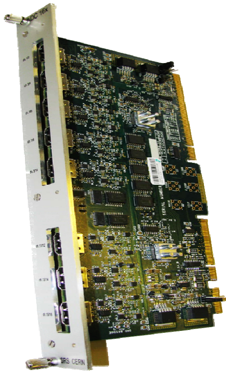
Fig. 8. Photo of the 6U SRS ADC adapter card for analog frontend chips.
