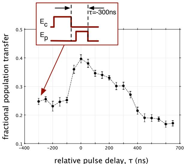
FIG. 4. (Color online) Demonstration of stimulated Raman adiabatic passage (STIRAP). For this test, we initialize the atoms to level  $|F = 1\rangle$  and probe the population of  $|F = 2\rangle$  as the overlap between the EIT pulses is varied. We observe maximal population transfer to  $|F = 2\rangle$  when the coupling and probe pulses completely overlap with coupling laser turning-on and turning-off before the probe laser beam.
