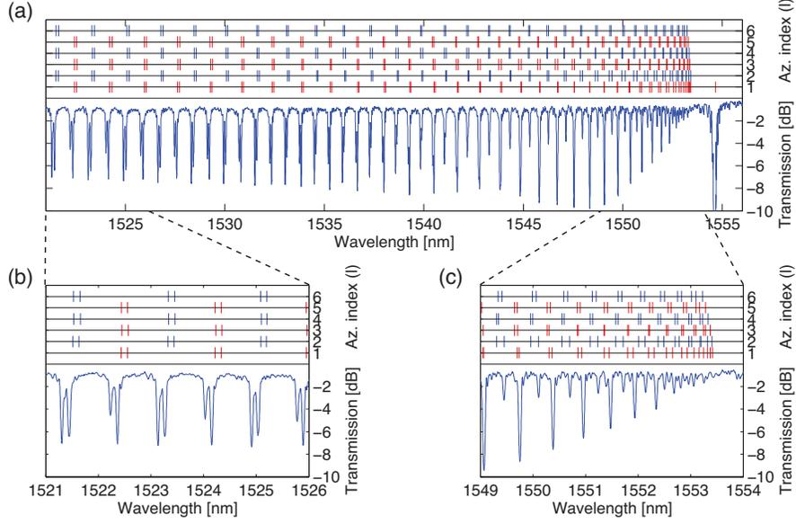
Fig. 4. Measured cladding mode spectra in transmission (bottom) and computed HE and EH resonances (top) for odd (red) and even (blue) azimuthal order  $l$ . (a) Complete measured wavelength range; (b) low- and (c) high-wavelength range in more detail.
