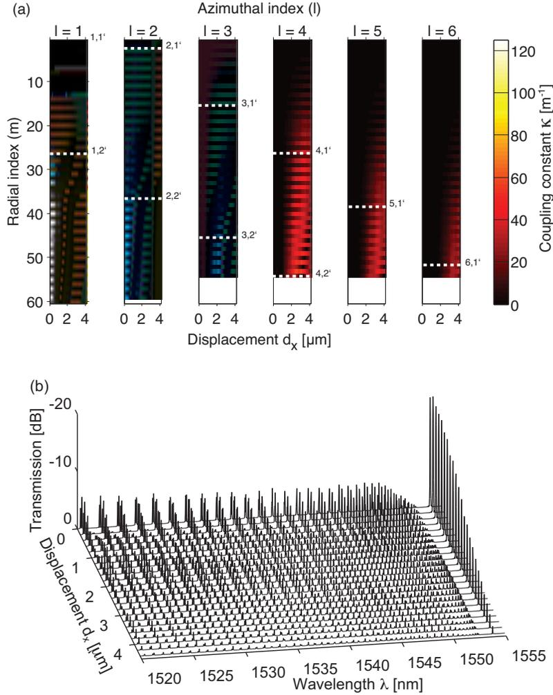
Fig. 5. (a) Core-cladding mode coupling coefficients for different displacements  $d_x$  of the microvoid in  $x$ -direction from the center of the fiber core. Coupling constants for  $l = 1$  to  $l = 6$  are plotted,  $m$  is ascending from top to bottom. Dotted lines indicate the virtual cutoffs. (b) Computed transmission spectra for different displacement of the modification in the  $x$ -direction.
