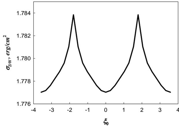
**Fig. 2** Dependence of the magnetic domain wall energy  $\sigma_{DW}$  on the parameter  $\zeta_0$  characterizing the displacement of the magnetic domain wall relative to the ferroelectric domain structure.
