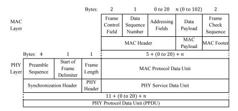
Fig. 2. Schematic view of the data frame [5]
