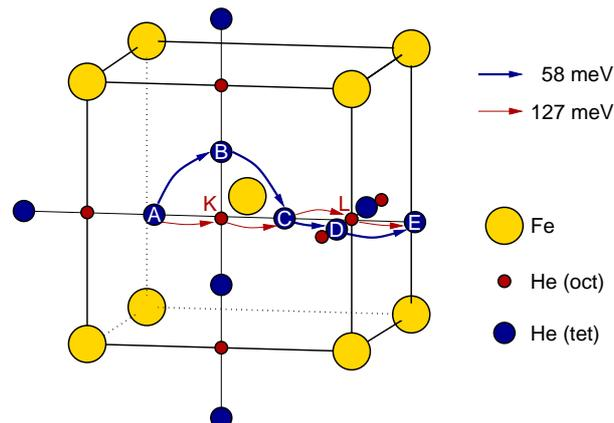
Figure A.5: Conventional unit cell of the body-centered cubic lattice illustrating the locations of tetrahedral and octahedral interstitial sites, and He migration barriers in the defect-free iron. Note that for clarity only a subset of the interstitial sites is shown.
