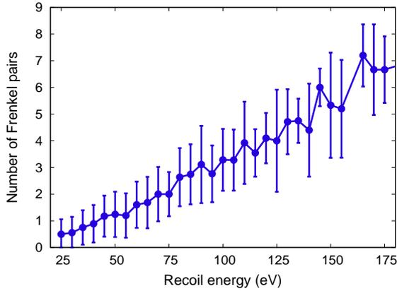
Figure 3: Average number of stable Frenkel pairs created during the MD simulations of He collision cascades in Fe. The bars indicate the standard deviation of the number of defects created.
