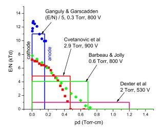
**Figure 2.** Measured (points) and approximate (lines) spatial distribution of electric field for Ganguly and Garscadden [12] - circles (blue), for Cvetanović *et al* [9] - squares (red), Barbeau and Jolly [11] - diamonds (green), and Dexter *et al* [48]. For the last three cases, the extent of the high-field region shown is equal to the stated cathode-fall thickness and the anode locations are well beyond the cathode fall.
