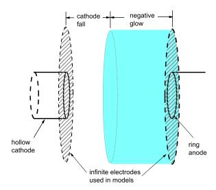
**Figure 1.** Schematic of low-pressure glow-discharge experiments analyzed in this paper, showing various electrode configurations discussed in the text.
