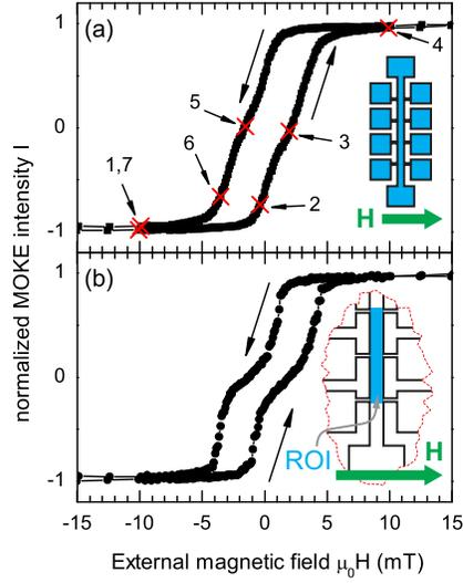
FIG. 3. (Color online) (a) MOKE intensity  $I$  integrated over the entire Hall bar and normalized to  $[-1,1]$  as a function of  $\mu_0 H$ . The numbers correspond to the MOKE images shown in Fig. 2. (b) Normalized  $I(H)$  integrated over the indicated region of interest (ROI). The two-step magnetic switching characteristic of cubic magnetic anisotropy is clearly evident from the data.
