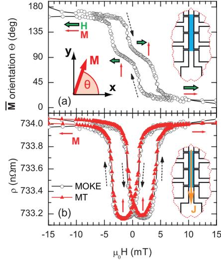
FIG. 4. (Color online) (a)  $\overline{\mathbf{M}}$  orientation  $\Theta(H)$  calculated from the integral MOKE intensity in the indicated region of interest. (b) The AMR calculated from  $\Theta(H)$  perfectly traces the experimentally observed  $R(H)$ .
