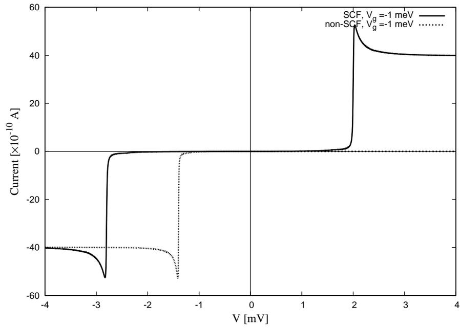
Figure 2: Zero temperature I-V characteristics calculated without the self consistent field (non-SCF) method (dashed curve) and calculated using the self consistent field (SCF) method (solid curve), with  $E_d = 0.2$  meV,  $V_g = -1$  meV,  $U_0 = 0.0025$  meV,  $C_D/C_E = 0.5$ ,  $\Gamma_L = \Gamma_R = 0.008$  meV and  $\Delta = 0.2$  meV.
