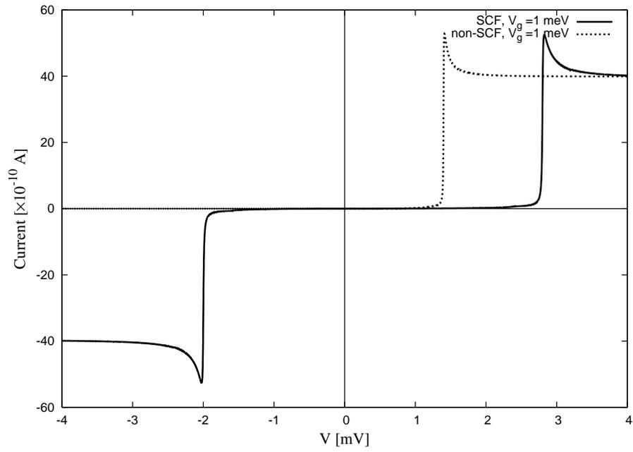
Figure 1: Zero temperature I-V characteristics calculated without the self consistent field (non-SCF) method (dashed curve) and calculated using the self consistent field (SCF) method (solid curve), with  $E_d = 0.2$  meV,  $V_g = 1$  meV,  $U_0 = 0.0025$  meV,  $C_D/C_E = 0.5$ ,  $\Gamma_L = \Gamma_R = 0.008$  meV and  $\Delta = 0.2$  meV.
