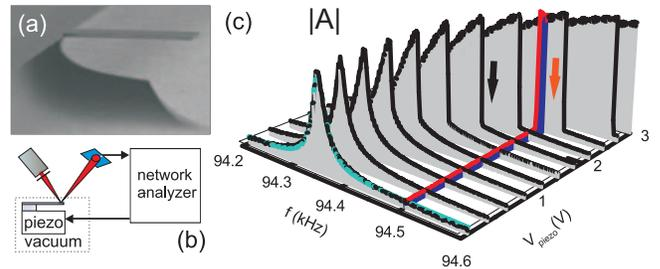
FIG. 1: (a) Scanning electron micrograph of a silicon nitride cantilever; (b) Experimental setup; (c) Response lines for several drive voltages (forward frequency sweeps). A damped driven harmonic oscillator fit is shown for the weakly driven cantilever. The line at  $f = 94.5 \text{kHz}$  represents a response along the (decreasing) drive strength axis. The arrows indicate the switching direction.
