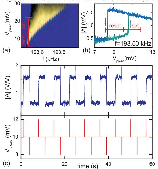
FIG. 3: Hysteretic regime for a  $30 \mu\text{m} \times 8 \mu\text{m} \times 150 \text{nm}$  cantilever. (b) Drive strength sweep at fixed frequency, and indication of the modulation to implement the bit. (c) Mechanical memory in a bistable cantilever beam: drive strength (lower panel) and cantilever response (upper panel).
