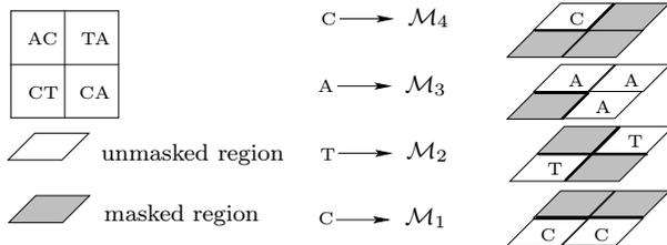
Figure 1: Asynchronous synthesis of a  $2 \times 2$  microarray. The deposition sequence  $D = CTAC$  corresponds to the sequence of four masks  $\mathcal{M}_1$ ,  $\mathcal{M}_2$ ,  $\mathcal{M}_3$ , and  $\mathcal{M}_4$ . The masked regions are shaded. The borders between the masked and unmasked regions are represented by bold lines. With respect to the deposition sequence  $D$ , the embedding of sequence AC is  $--AC$ , TA is  $-TA-$ , CT is  $CT--$ , CA is  $C-A-$ .
