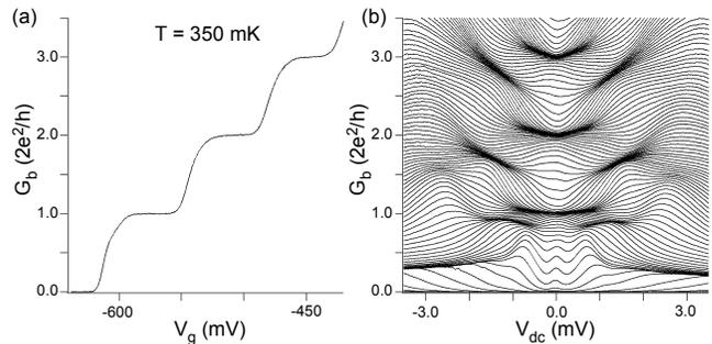
FIG. 6: Conductance data of QPC without tip. (a) Conductance plateaus as a function of  $V_g$ , which controls the number of transmitting sub-bands. (b)  $G_b(V_{dc})$  for small steps in  $V_g$  (i.e.  $G_b(V_{dc}, V_g)$ ) for the  $L = 4.0$   $\mu\text{m}$  measurement in Fig. 3(a). The data have been corrected for series resistance leading to the QPC.
