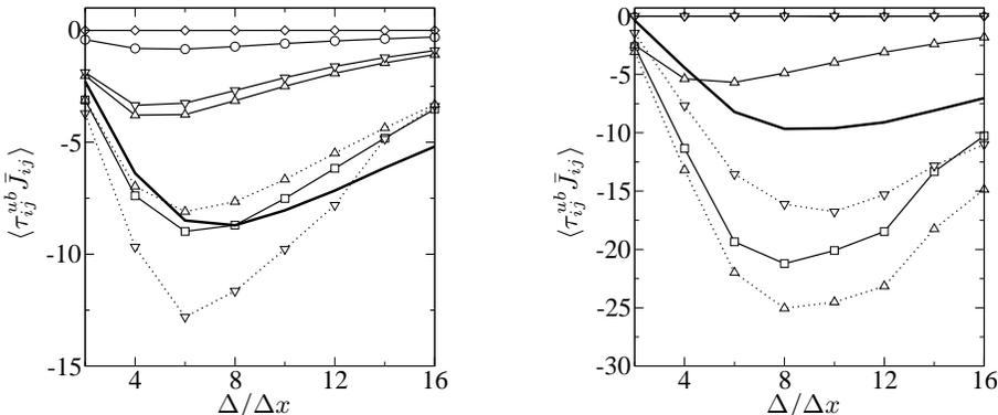
FIGURE 3. Functional performance of models. Evolution of the mean GS/SGS magnetic energy transfer with the filter size for box (left) and spectral cutoff (right) filter (see Table 2.1 for symbols correspondence). The thick line is the mean GS/SGS magnetic energy transfer from the filtered DNS.
