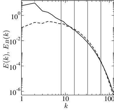
FIGURE 1. Kinetic,  $E(k)$ , and magnetic,  $E_B(k)$ , energy spectra:  $E(k)$  — ;  $E_B(k)$  ---- . The thin vertical lines show the location of some filters used in this work:  $\Delta/\Delta x = 2, 4, 8$  and 16.
