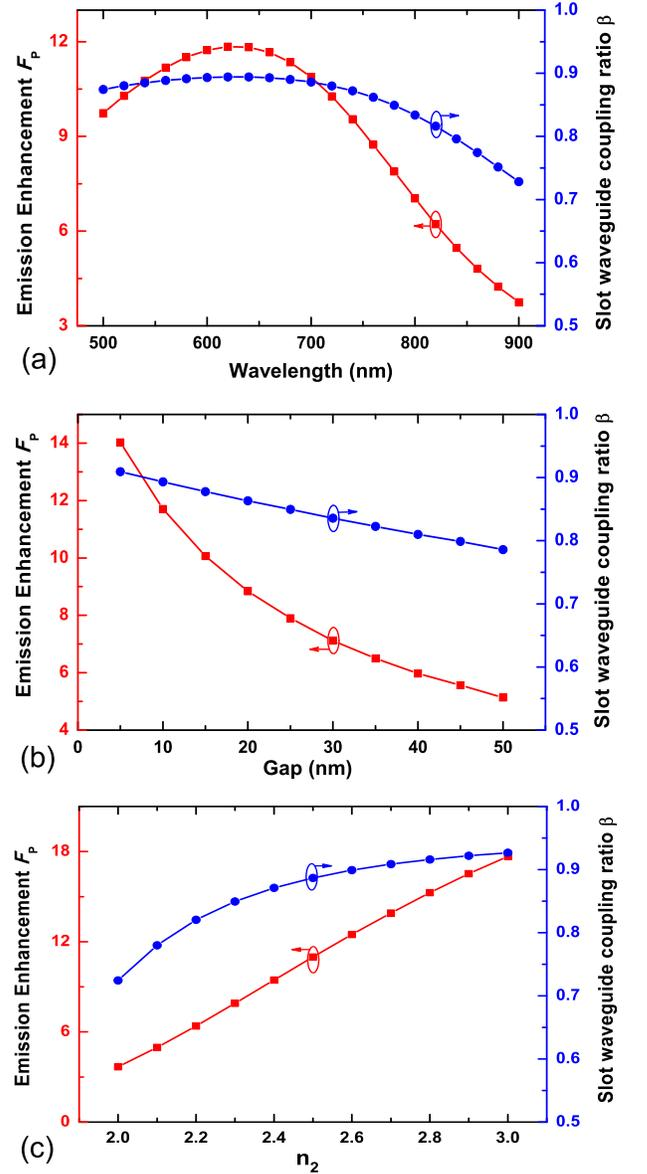
FIG. 3: (a) Spontaneous emission enhancement ( $F_p$ ) and waveguide coupling efficiency ( $\beta$ ) depending on the working wavelength for slot waveguides with  $g = 10$  nm. (b)  $F_p$  and  $\beta$  depending on the slot width (gap)  $g$  with  $\lambda = 650$  nm. In all cases,  $a = 100$  nm,  $b = 150$  nm. (c)  $F_p$  and  $\beta$  depending on  $n_2$  with  $\lambda = 550$  nm,  $g = 10$  nm. In all cases,  $a = 100$  nm,  $b = 150$  nm.
