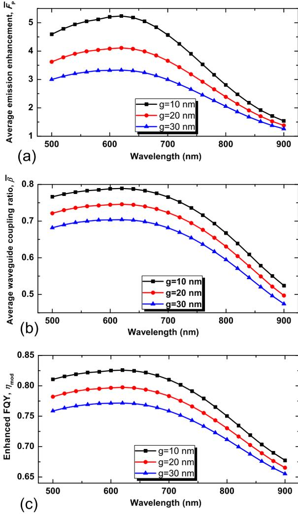
FIG. 4: (a), (b) Average spontaneous emission enhancement ( $\overline{F}_p$ ) and average waveguide coupling efficiency ( $\overline{\beta}$ ) depending on the working wavelength for slot waveguides, respectively. (c) The enhanced FQY  $\eta$  as a function of wavelength with initial FQY  $\eta_0 = 0.5$ . In all cases,  $a = 100$  nm,  $b = 150$  nm.
