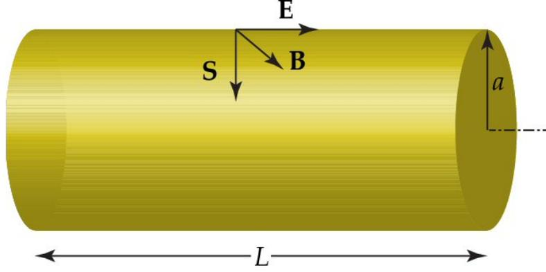
FIG. 1: Variables defined for calculation of energy dissipated in a wire.
