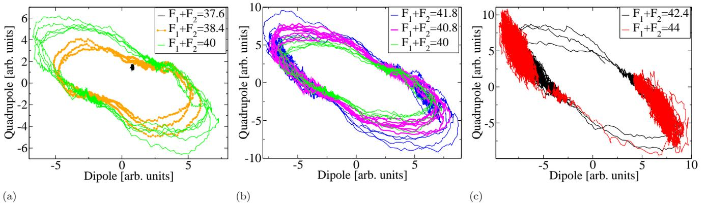
FIG. 4: (Color online) (a): Evolution of the magnetic field in the phase space ( $D, Q$ ) at low frequencies: there exists a range of bistability in which a stationary dynamo (black dot) and a periodic limit cycle (orange circles) are both metastable. (b): Evolution of the limit cycle when  $F_1 + F_2$  is increased from 40 to 41.8 Hz. (c): Chaotic reversals obtained for large values of  $F_1 + F_2$  in the vicinity of a saddle-node bifurcation.
