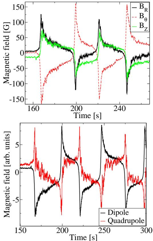
FIG. 3: (Color online) Top: time recordings of the three components of the magnetic field. The rotation frequencies are increased from 14.4/24 Hz to 15/25 Hz, leading to a transition from a stationary low amplitude dynamo regime to a limit cycle. Bottom: Behavior of the dipolar and quadrupolar parts of the magnetic field. Note the transfer between the two components during reversals.
