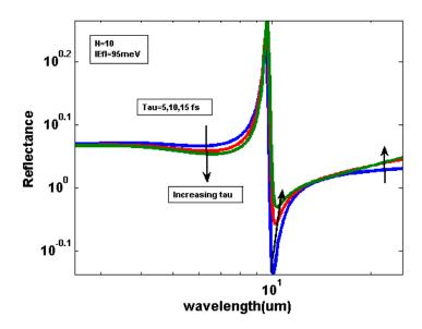
Fig1(c): Variation of Reflection of graphene for various  $\tau$  where N= 10 and IE<sub>F</sub>I=95meV.
