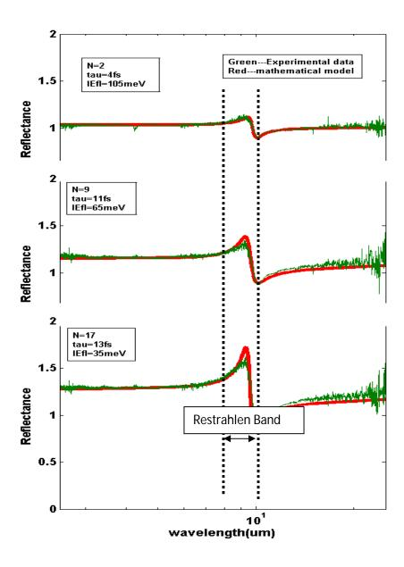
Fig3: Measured reflection spectra (green line) from  $2.5\mu m$  to  $25\mu m$  along with theoretical reflection spectra (red line) using eqs. (1)-(4) considering complex dielectric constant for SiC.
