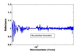
Fig2b(I): Reflection spectrum of SiC substrate
