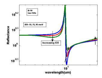
Fig1(a): Variation of Reflection of graphene for various N where IE<sub>F</sub>I=95meV and  $\tau$ =15fs.
