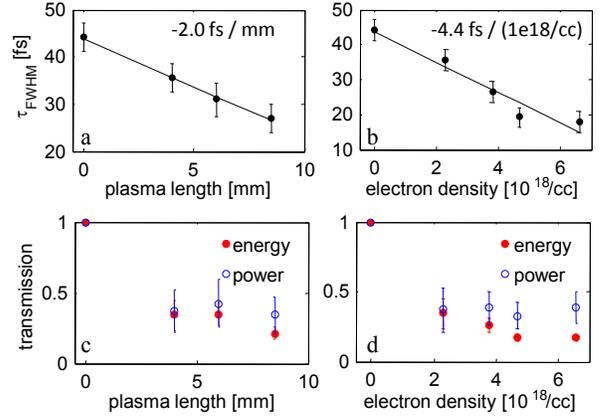
FIG. 3: (color online) Dependence of pulse duration  $\tau$  on (a) propagation length  $l$  for  $n_e = (1.2..2.3) \times 10^{18} \text{cm}^{-3}$  and (b) electron density  $n_e$  for  $l = 4$  mm. Best fit lines give compression rates of 2.0 fs/mm and 4.4 fs/( $10^{18} \text{cm}^{-3}$ ) respectively. (c), (d) shows transmission in terms of laser energy (full circles) and peak power (open).
