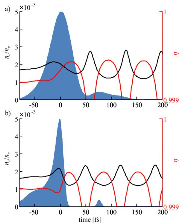
FIG. 4: (color online) Numerical solution of 1D wave equation in quasistatic approximation.  $a^2$  (blue filled),  $n_e$  (black solid), and  $\eta$  (red) resulting from propagation of a pulse with  $a_0 \simeq 1.5$  at  $n_{e0} = 2.5 \times 10^{18}\text{ cm}^{-3}$ ; (a) initially, (b) at  $l = 8\text{ mm}$ . The reduced  $a_0$  was chosen to account for the initial energy loss in the guided mode as in Fig. 3.
