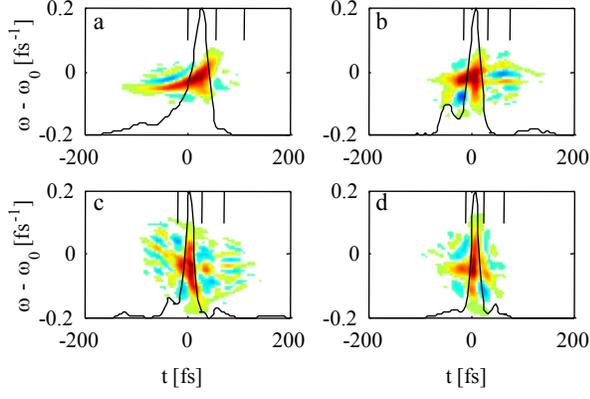
FIG. 2: (color online) Pulse profiles for  $n_e =$  (a) 2.3, (b) 3.8, (c) 4.7, and (d)  $6.6 \times 10^{18} \text{cm}^{-3}$  for  $l = 4$  mm. The black vertical lines mark the plasma period ( $2\pi/\omega_p$ ), i.e. expected positions of electron density maxima for the respective densities.
