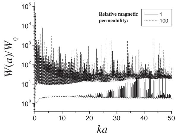
Figure 3: The normalized time-averaged internal energy  $W(a)/W_0$  plotted as a function of the size parameter  $ka$ . The values of the relative permeability are  $\mu_1/\mu = 1$  (nonmagnetic sphere) and  $\mu_1/\mu = 100$  (magnetic sphere). The relative refraction index is  $m = 1.334 + 1.5 \times 10^{-9}i$ , which have been used in [17] in the nonmagnetic scattering approach. The quantities are calculated in the interval  $1 \leq ka \leq 50$ ,  $\delta(ka) = 0.01$ .
