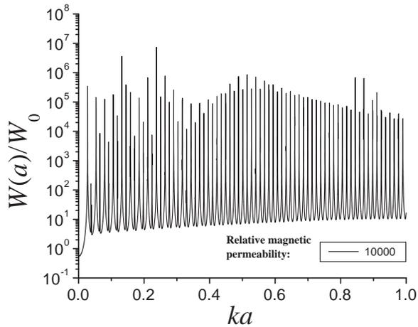
Figure 2: The normalized time-averaged internal energy  $W(a)/W_0$  within a non-absorptive magnetic sphere plotted as a function of the size parameter  $ka$ . The values of the relative permittivity and permeability are  $\epsilon_1/\epsilon = 1.4161$  and  $\mu_1/\mu = 10^4$ , respectively. The internal energy  $W(a)/W_0$  is calculated in the interval  $10^{-6} \leq ka \leq 1$ ,  $\delta(ka) = 10^{-4}$ .
