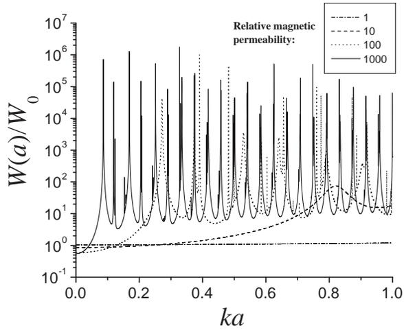
Figure 1: Comparison among the distributions of  $W(a)/W_0$  in function of the size parameter  $ka$ . The values of the relative permittivity and permeability related to a non-absorptive sphere are  $\epsilon_1/\epsilon = 1.4161$  and  $\mu_1/\mu = 1, 10, 100, 1000$ , respectively. The internal energy  $W(a)/W_0$  is calculated in the interval  $10^{-6} \leq ka \leq 1$ ,  $\delta(ka) = 10^{-4}$ .
