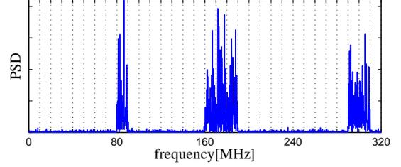
**Fig. 1.** Spectrum of a wideband signal received at the sensing radio with  $L = 32$  total bands and  $N = 6$  active channels. The active channel set is  $\mathbf{b} = [8, 16, 17, 18, 29, 30]$ .
