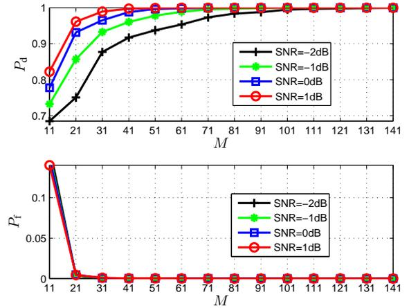
**Fig. 6.** Detection performance of the proposed model versus  $M$  and SNR for the simulated wideband system..
