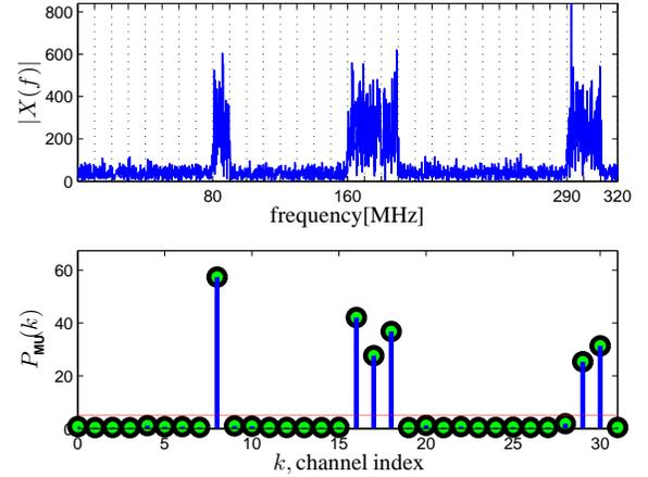
**Fig. 4.** Frequency representation,  $X(f)$ , and the corresponding  $P_{MU}$  values of a typical wideband signal with  $L = 32$  channels. The position of six significant values specify the occupied channels  $\hat{\mathbf{b}} = [8, 16, 17, 18, 29, 30]$ .
