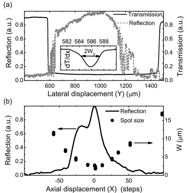
FIG. 3. (a) Reflected and transmitted signal as a function of the lateral position ( $y$ -axis) of the sample. The spot size  $W$  of the beam on the sample surface (waist  $W_0$  when in focus) is determined with the knife-edge technique (inset). (b) Reflected signal (solid line) and the spot size  $W$  (dots) as a function of the axial displacement ( $x$ -axis) of the sample.
