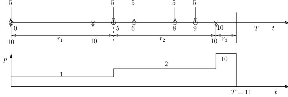
Fig. 10. Optimal transmit powers  $\mathbf{p} = [1, 2, 10]$ mW, with durations  $\mathbf{l} = [5, 5, 1] \times 10^{-2}$ s.
