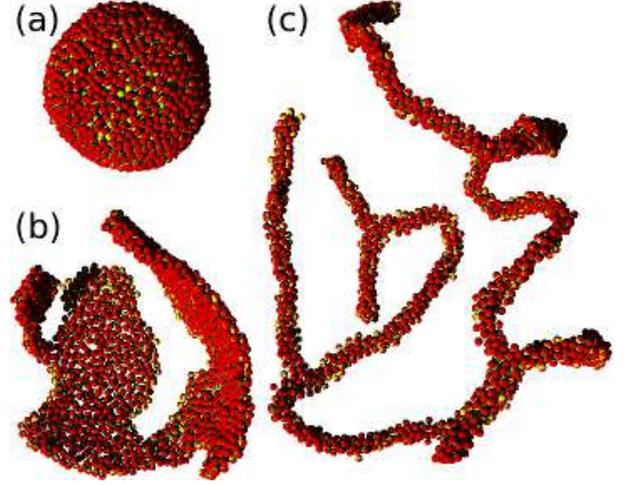
FIG. 19: (Color online) Sequential snapshots of vesicle rupture at  $N = 2000$ ,  $\epsilon = 2$ ,  $\rho^* = 14$ ,  $k_{bend} = 8$ ,  $k_{tilt} = 8$ , and  $C_{bd} = 0.85$ . (a)  $t/\tau_0 = 500$ . (b)  $t/\tau_0 = 640$ . (c)  $t/\tau_0 = 3000$ .
