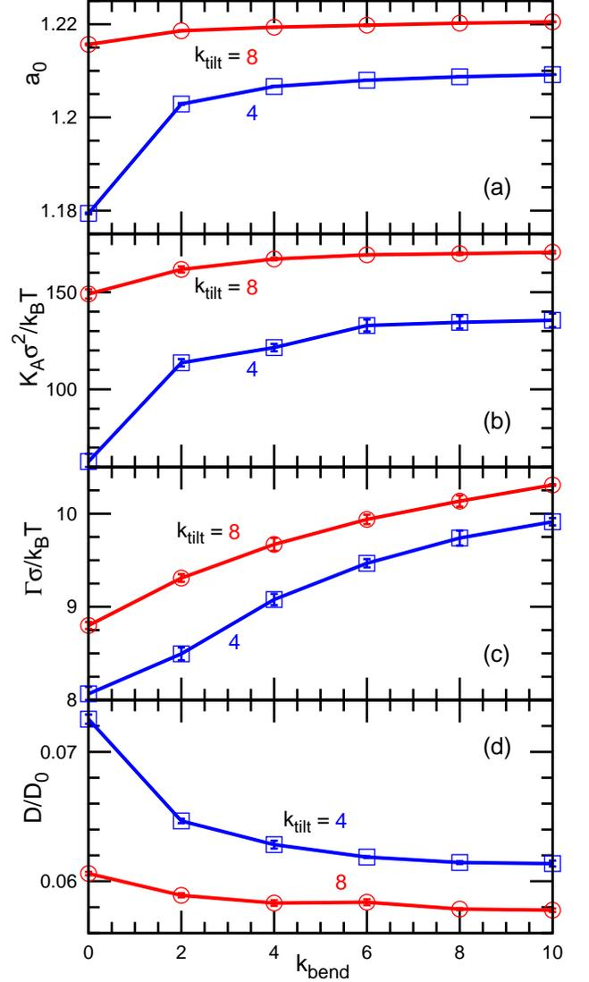
FIG. 15: (Color online) Parameter  $k_{\text{bend}}$  dependence of (a)  $a_0 = 2A_0/N\sigma^2$ , (b)  $K_A$ , (c)  $\Gamma$ , and (d)  $D$  for  $\rho^* = 14$ ,  $\varepsilon = 2$ , and  $C_{\text{bd}} = 0$ . The squares and circles represent data for  $k_{\text{tilt}} = 4$  and  $8$ , respectively.
