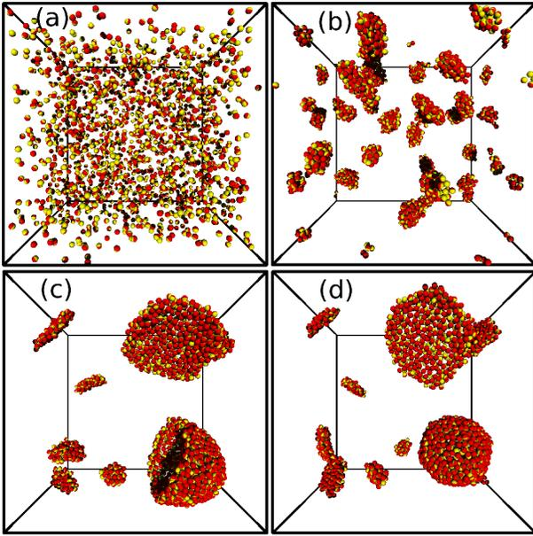
FIG. 3: (Color online) Sequential snapshots of the molecular self-assembly at  $N = 2000$ ,  $L_x = L_y = L_z = 40\sigma$ ,  $\varepsilon = 2$ ,  $\rho^* = 14$ ,  $k_{\text{bend}} = 0$ ,  $k_{\text{tilt}} = 8$ , and  $C_{\text{bd}} = 0$ . (a)  $t/\tau_0 = 0$ . (b)  $t/\tau_0 = 500$ . (c)  $t/\tau_0 = 16650$ . (d)  $t/\tau_0 = 16700$ .
