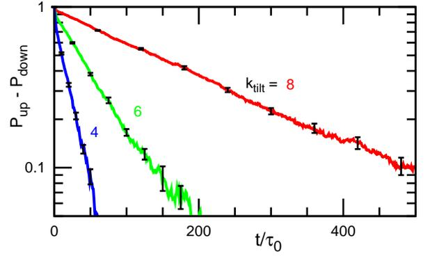
FIG. 10: (Color online) Time development of the probability difference  $P_{\text{up}} - P_{\text{down}}$  of the molecules in the upper and lower monolayers at  $N = 512$ ,  $\rho^* = 14$ ,  $\varepsilon = 2$ ,  $k_{\text{bend}} = 0$ , and  $C_{\text{bd}} = 0$ . At the initial states ( $t = 0$ ),  $P_{\text{up}} = 1$  and  $P_{\text{down}} = 0$ . The error bars are displayed at several data points.
