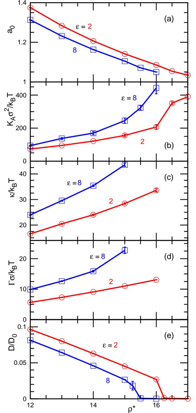
FIG. 11: (Color online) Parameter  $\rho^*$  dependence of (a) the intrinsic area  $a_0 = 2A_0/N\sigma^2$  per molecule, (b) area compression modulus  $K_A$ , (c) bending rigidity  $\kappa$ , (d) line tension  $\Gamma$ , and (e) diffusion coefficient  $D$  for the tensionless membrane at  $k_{\text{tilt}} = 4$ ,  $k_{\text{bend}} = 4$ , and  $C_{\text{bd}} = 0$ . The circles and squares represent data for  $\varepsilon = 2$  and  $8$ , respectively.
