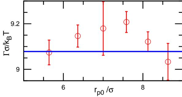
FIG. 9: (Color online) Line tension  $\Gamma$  of membrane edge at  $\varepsilon = 2$ ,  $\rho^* = 14$ ,  $k_{\text{bend}} = 4$ ,  $k_{\text{tilt}} = 4$ , and  $C_{\text{bd}} = 0$ . The circles represent  $\Gamma$  calculated from a pore on the flat membrane at  $N = 2048$ . The solid line represents  $\Gamma$  calculated from the striped membrane at  $N = 512$ :  $\Gamma\sigma/k_B T = 9.08 \pm 0.06$ .
