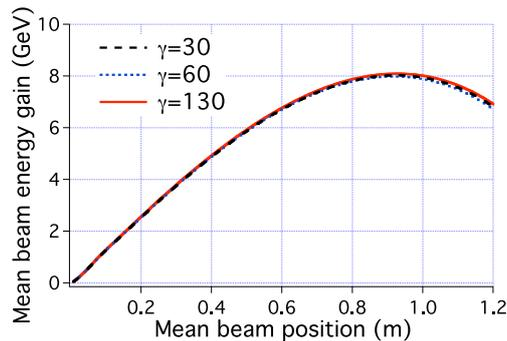
Figure 19: Average beam energy gain versus longitudinal position (in the laboratory frame) from 2D-1/2 simulations of a full scale 10GeV LPA in a boosted frame at  $\gamma = 30, 60$  and 130, using the Yee solver.
