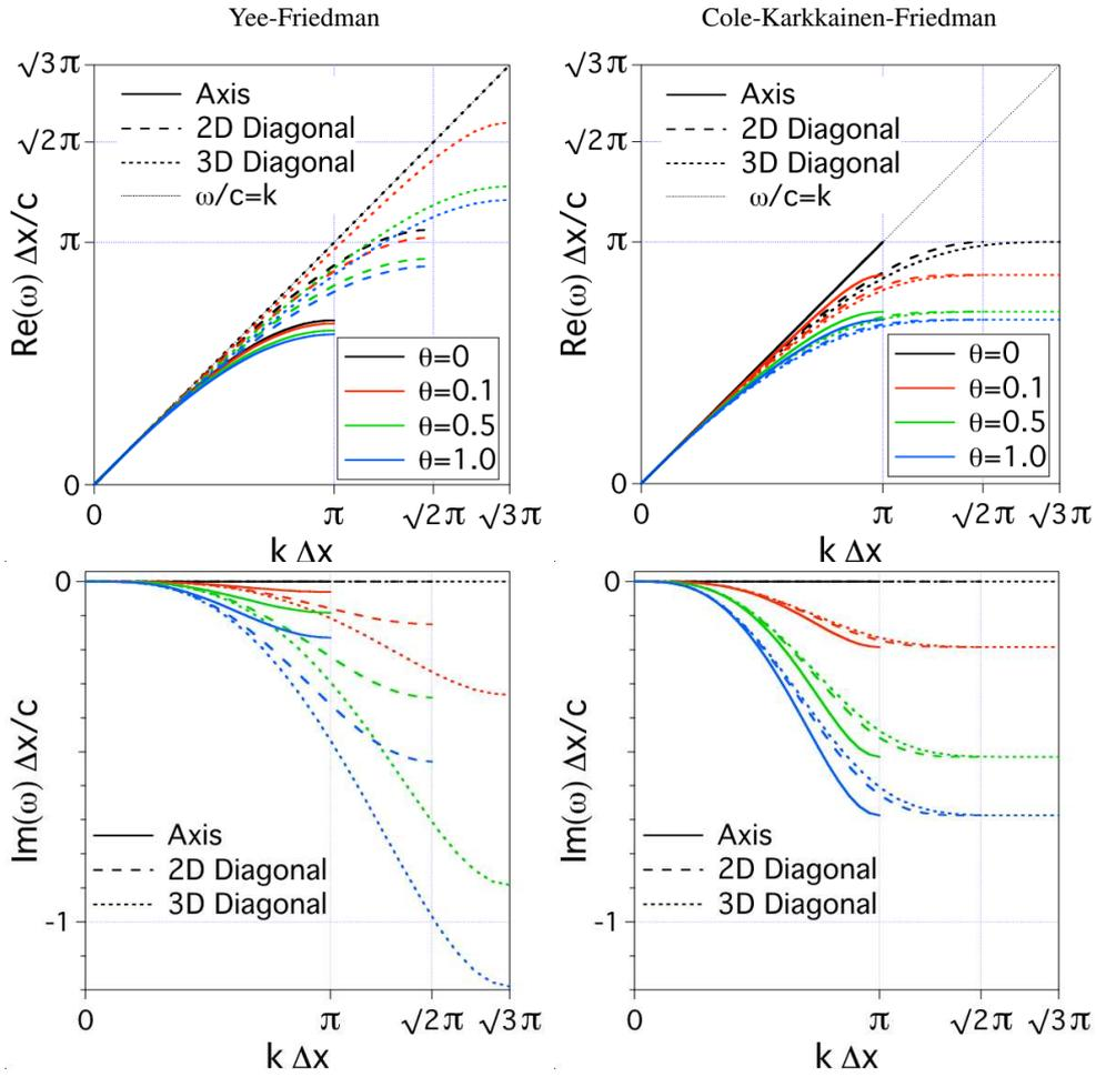
Figure 8: Numerical dispersion along the principal axis and diagonals for cubic cells ( $\delta x = \delta y = \delta z$ ) at the Courant limit for: (left) the Yee-Friedman solver; (right) the Cole-Karkkainen-Friedman solver. The real part (phase) and the imaginary part (amplitude) are plotted respectively in the top and bottom rows.
