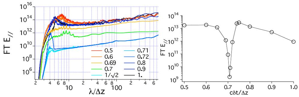
Figure 26: Fourier Transform of the longitudinal electric field at  $t=40$  ps, averaged over the whole domain, from 2-1/2D simulations of a full scale 10GeV LPA in a boosted frame at  $\gamma = 130$ , using the CK solver, for time steps between  $c\delta t/\delta z = 0.5$  and  $c\delta t/\delta z = 1$ , versus  $\lambda/\delta z$  (left) and at  $\lambda/\delta z = 4$  (right).
