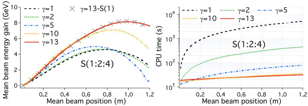
Figure 15: (left) Average scaled beam energy gain and (right) CPU time, versus longitudinal position in the laboratory frame from simulations in the laboratory frame ( $\gamma = 1$ ) and boosted frames at  $\gamma = 2, 5, 10$  and  $13$ , using the Yee solver with digital filter S(1:2:4) (grey cross is reference from run with filter S(1)).
