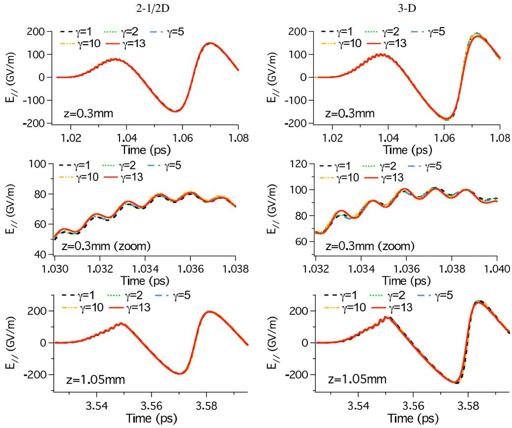
Figure 12: History of longitudinal electric field at the position  $x = y = 0$ ,  $z = 0.3$  mm and  $z = 1.05$  mm (in the laboratory frame) from simulations in the laboratory frame ( $\gamma = 1$ ) and boosted frames at  $\gamma = 2, 5, 10$  and  $13$ .
