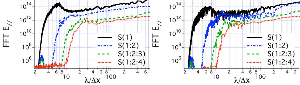
Figure 23: Fourier Transform of the longitudinal electric field at  $t=40$  ps, averaged over plane on axis perpendicular to laser polarization, from (left) 3D and (right) 2D-1/2 simulations of a full scale 10GeV LPA in a boosted frame at  $\gamma = 130$ , using the Yee solver and various smoothing kernels. The same time step at the 3D CFL limit  $c\delta t = \delta x / \sqrt{3}$  was used for both simulations.
