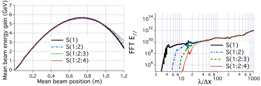
Figure 21: (left) Average beam energy gain versus longitudinal position (in the laboratory frame), (right) Fourier Transform of the longitudinal electric field at  $t=40$  ps, averaged over whole domain, from 3D simulations of a full scale 10GeV LPA in a boosted frame at  $\gamma = 130$ , using the CK2 solver and various digital filter kernels.
