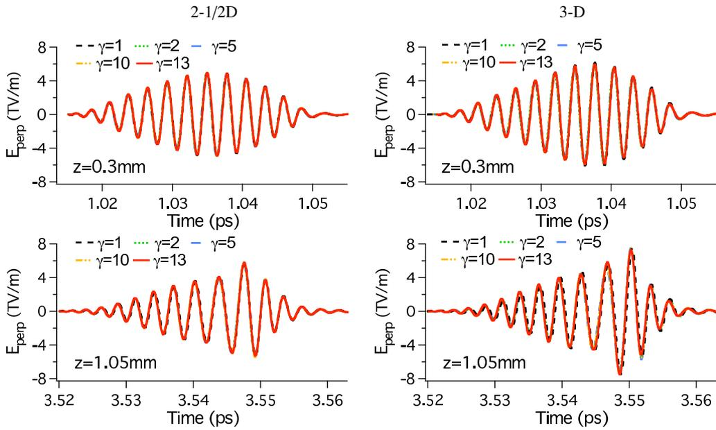
Figure 11: History of transverse electric field at the position  $x = y = 0$ ,  $z = 0.3 \text{ mm}$  and  $z = 1.05 \text{ mm}$  (in the laboratory frame) from simulations in the laboratory frame ( $\gamma = 1$ ) and boosted frames at  $\gamma = 2, 5, 10$  and  $13$ .
