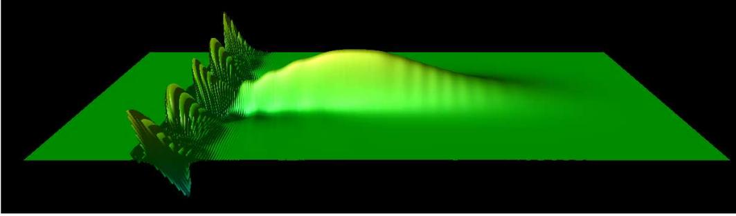
Figure 3: Snapshot of a surface plot of the longitudinal field from a 2-1/2D simulation of a full scale 10GeV LPA in a boosted frame at  $\gamma = 130$  (elevation is proportional to the magnitude of the electric field). The laser is propagating from left to right and the plasma from right to left. A fast growing short wavelength instability is developing at the front of the plasma.
