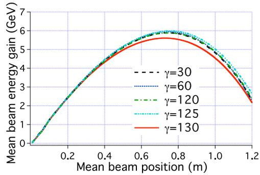
Figure 22: Average beam energy gain versus longitudinal position (in the laboratory frame) from 3D simulations of a full scale 10GeV LPA in a boosted frame at  $\gamma = 30, 60, 120, 125$  and  $130$ , using the Yee solver ( $\gamma = 30$  and  $60$ ) and the CK2 solver ( $\gamma = 120 - 130$ ), with digital filter S(1) and with the time step set by  $c\delta t/\delta z = 1/\sqrt{2}$  for stability (see discussion below).
