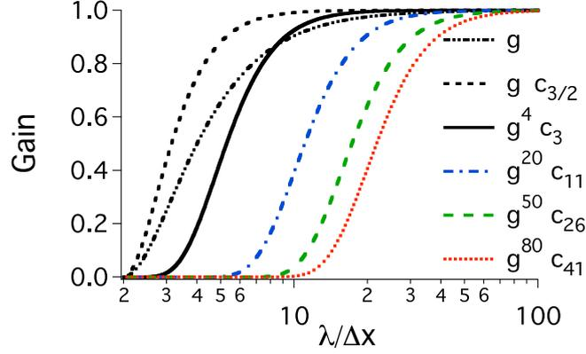
Figure 4: Gain versus wavelength for the bilinear filter without compensation ( $g = g(1/2, k)$ ), with compensation ( $g \cdot c_{3/2} = g(1/2, k) \cdot g(3/2, k)$ ), and  $n$ -pass bilinear filters with compensation ( $g^n \cdot c_{\alpha_c} = g(1/2, k)^n \cdot g(\alpha_c, k)$ ) for  $n = 4, 20, 50$  and  $80$ .
