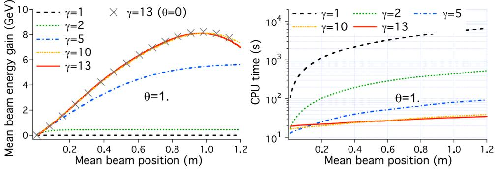
Figure 17: (left) Average scaled beam energy gain and (right) CPU time, versus longitudinal position in the laboratory frame from simulations in the laboratory frame ( $\gamma = 1$ ) and boosted frames at  $\gamma = 2, 5, 10$  and  $13$ , using the Yee-Friedman solver with  $\theta = 1$  (grey cross is reference from run with no damping).
