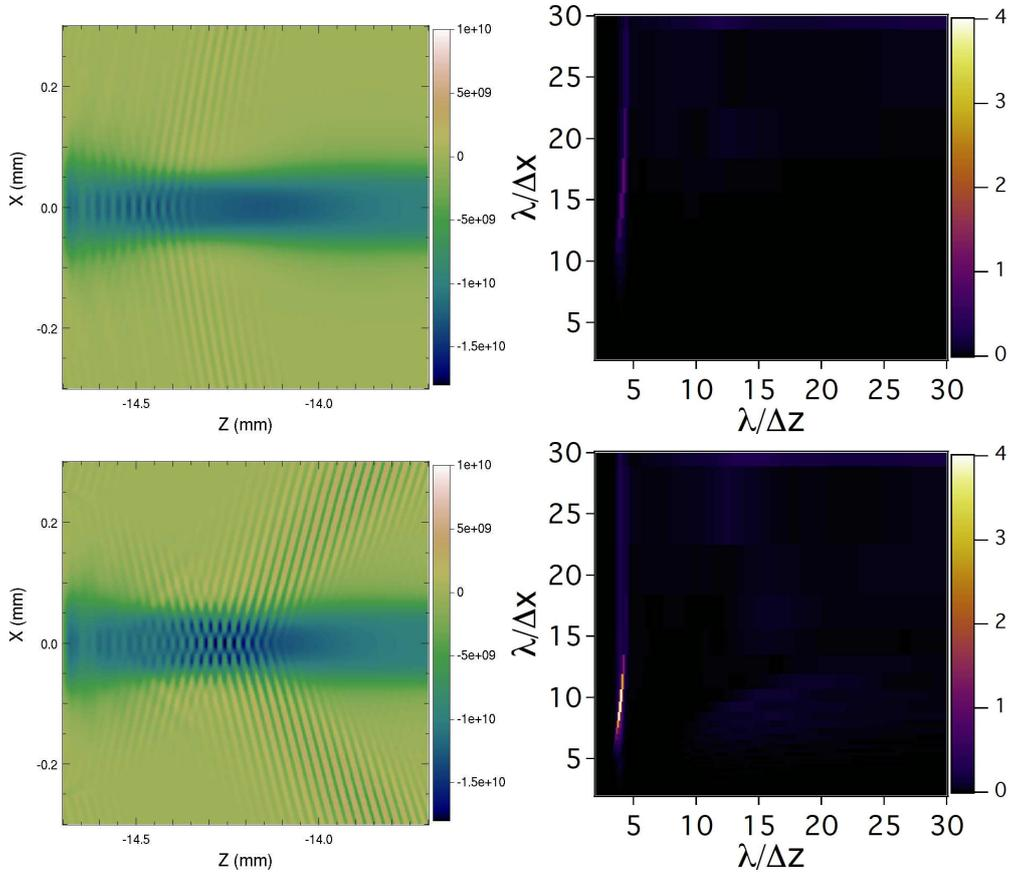
Figure 27: (left) Snapshot of the longitudinal electric field ( $E_{||}$ ) at the front of the plasma at  $t = 49$  ps; (right) Fourier Transform of the longitudinal electric field, from 2-1/2D simulations of a full scale 10GeV LPA in a boosted frame at  $\gamma = 130$ , using  $\delta_x = \delta_z = 6.5\mu\text{m}$ , and the time step at the 2D CFL limit  $c\delta t = \delta z/\sqrt{2}$ , for (top) the Yee solver; (bottom) the CK solver.
