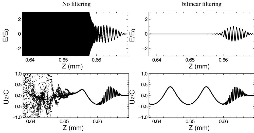
Figure 32: Snapshots from transverse electric field (normalized to maximum laser amplitude  $E_0$ ) and plasma electrons longitudinal phase space projection, from a 1D simulation of a laser wakefield acceleration stage the CFL limits ( $c\delta t = \delta x$ ) with (left) no filtering of current density; (right) application of a bilinear digital filter to the current density.
