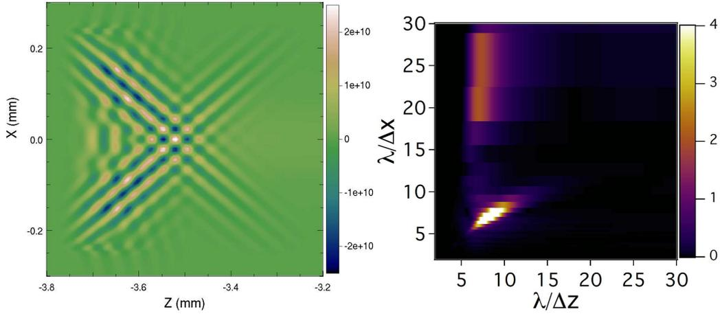
Figure 25: (left) Snapshot of the longitudinal electric field ( $E_{//}$ ) at the front of the plasma at  $t = 12.5$  ps; (right) Fourier Transform of the longitudinal electric field, from 2-1/2D simulations of a full scale 10GeV LPA in a boosted frame at  $\gamma = 130$ , with the CK solver, using  $\delta x = \delta z = 6.5\mu m$ , and the time step at the 3D CFL limit  $c\delta t = \delta x/\sqrt{3}$ .
