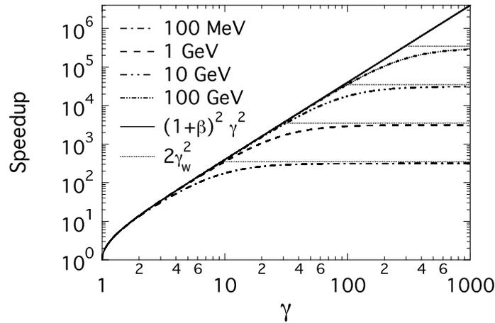
Figure 1: Speedup versus relativistic factor of the boosted frame from Eq.(13) for 100 MeV - 100 GeV LPA class stages.
