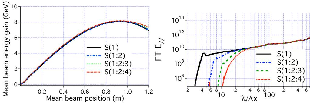
Figure 18: (left) Average beam energy gain versus longitudinal position (in the laboratory frame), (right) Fourier Transform of the longitudinal electric field at  $t=40$  ps, averaged over whole domain, from 2D-1/2 simulations of a full scale 10GeV LPA in a boosted frame at  $\gamma = 130$ , using the Yee solver and various digital filter kernels. Square cells ( $\delta x = \delta z = 6.5 \mu\text{m}$ ) and the CFL time step ( $c\delta t/\delta z = 1/\sqrt{2}$ ) were used.
