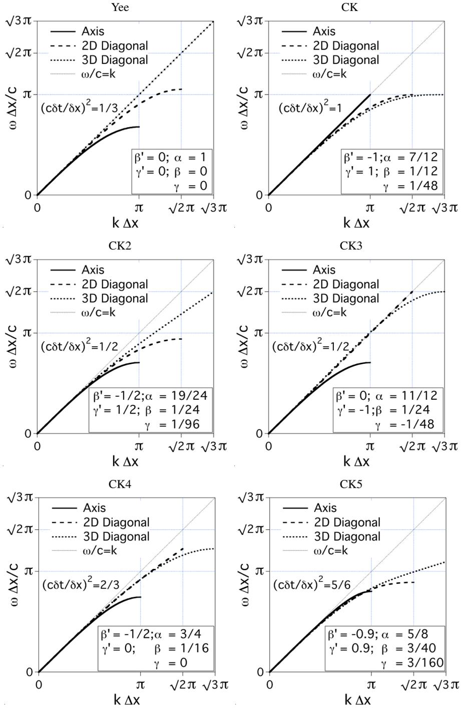
Figure 7: Numerical dispersion along the principal axis and diagonals for cubic cells ( $\delta x = \delta y = \delta z$ ) at the Courant limit for the solver with adjustable numerical dispersion using the parameters from Table 1.
