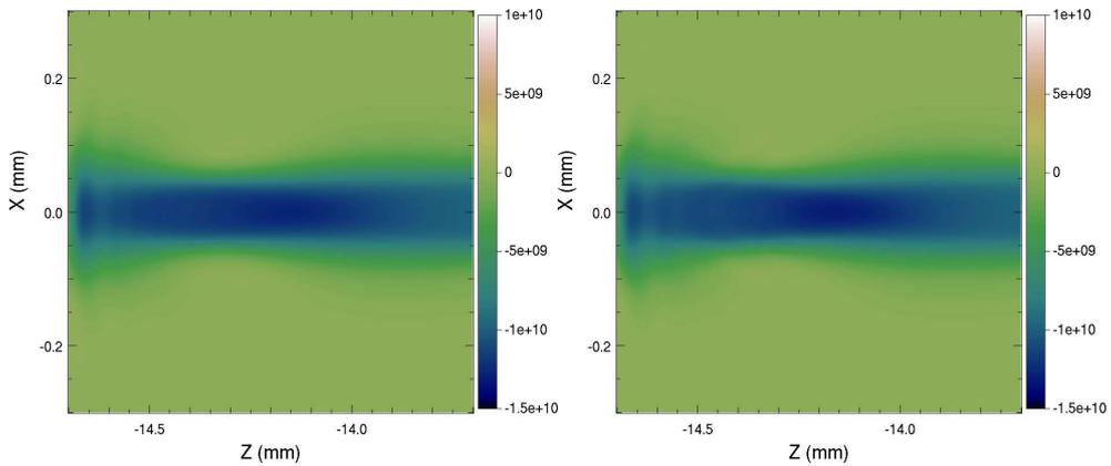
Figure 28: Snapshot of the longitudinal electric field ( $E_{||}$ ) at the front of the plasma at  $t = 49$  ps from 2-1/2D simulations of a full scale 10GeV LPA in a boosted frame at  $\gamma = 130$ , using  $\delta_x = \delta_z = 6.5\mu\text{m}$ , and the time step at the 2D CFL limit  $c\delta t = \delta z/\sqrt{2}$ , for (left) the Yee solver; (right) the CK solver. The filter S(1:2) was used to remove the instability that is visible in Fig. 27. The remaining feature is the wake.
