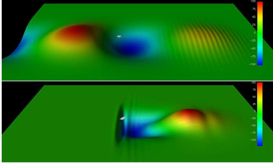
Figure 10: Colored surface rendering of the longitudinal electric field from a 2-1/2D Warp simulation of a laser wakefield acceleration stage in the laboratory frame (top) and a boosted frame at  $\gamma = 13$  (bottom), with the beam (white) in its early phase of acceleration. The laser and the beam are propagating from left to right.
