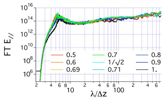
Figure 29: Fourier Transform of the longitudinal electric field at  $t=40$  ps, averaged over the whole domain, from 2-1/2D simulations of a full scale 10GeV LPA in a boosted frame at  $\gamma = 130$ , using the CK solver, for time steps between  $c\delta t/\delta z = 0.5$  and  $c\delta t/\delta z = 1$ , using a 'momentum conserving' field gathering scheme.
