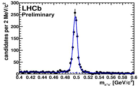
Figure 1: Invariant mass distribution for  $K_S^0 \rightarrow \pi^+\pi^-$  candidates as reconstructed from *long* tracks after selection. Beam-gas interactions have been statistically subtracted from this distribution.
