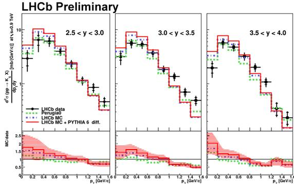
Figure 2: Double differential prompt  $K_S^0$  production cross-section in  $pp$  collisions at  $\sqrt{s} = 0.9$  TeV. Data are presented as three transverse momentum distributions in three bins of rapidity. LHCb preliminary results are marked by black dots: error bars represent statistical uncertainties while thick bars represent the systematic ones. Data are compared to predictions from different settings of the PYTHIA generator [1, 4]. Bottom plots show MC to data ratios.
