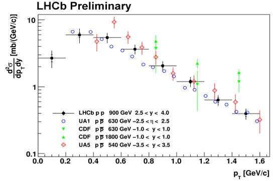
Figure 3: Comparison of double differential  $K_S^0$  production cross-section measurements obtained by the LHCb, CDF [7], UA1 [8], UA5 [9] experiments in different rapidity ( $y$ ) or pseudorapidity ( $\eta$ ) ranges.
