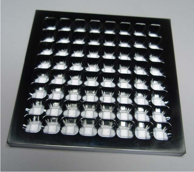
Figure 1: Photograph of the light concentrator. The chrome-plated 4.5 mm thick brass plate contains 64 pyramid-shaped funnels with quadratic (rounded edges) entrance and exit apertures of 7 \times 7 \text{ mm}^2 and 3 \times 3 \text{ mm}^2 , respectively.
