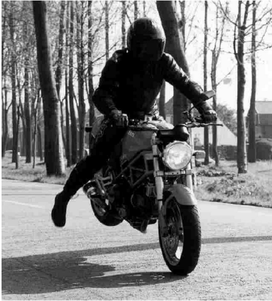
Figure 5. Braking of a motorcycle with maximum deceleration.
