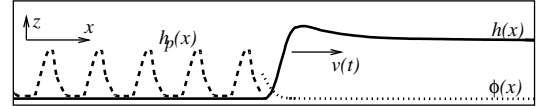
FIG. 1: Sketch of a liquid front that recedes due to evaporation and convection with a varying velocity v(t) . The deposition process is characterized by the film thickness profile h(x, t) , the concentration profile \phi(x, t) (in the bulk film), and the particle layer thickness h_p(x, t) = \phi(x, t)h(x, t) (outside the bulk film).
