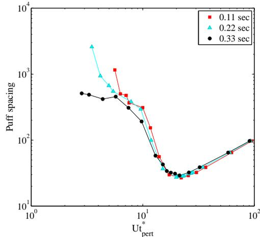
FIG. 4: Impact of valve opening time on puff spacings. Three different valve timings (0.11, 0.22 & 0.33 sec) were used. In the x-axis  $t_{pert}^*$  is the time between pulses taking valve opening time into account (see text)
