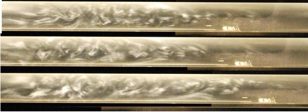
FIG. 2: Flow visualisation images of a turbulent puff at  $Re = 2000$  at 50 D (top), 100 D (middle) and 150 D (bottom) from the point of perturbation. Flow direction is from left to right. The puff reaches its typical size in less than 50 D from the perturbation point and the size is constant except for statistical fluctuations.
