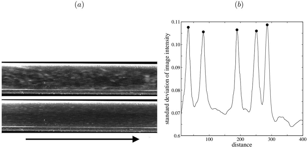
FIG. 6: (a) Flow visualization at  $Re = 2000$  in turbulent (upper image) and laminar flow (lower image). Images display a pipe segment of 5-6  $D$  long. Flow direction is from left to right. One reduction experiment is shown in movie 1 available in the online version of the paper. (b) Standard deviation of image intensity vs. reconstructed pipe position at  $Re = 2100$ . Summits of the peaks (black dots) indicate the position of a turbulent spot.
