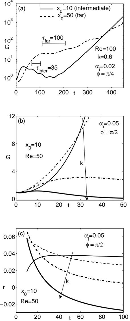
Figure 2: (a) The amplification factor  $G$ , asymmetric initial condition, intermediate ( $x_0 = 10$ , solid curves) and far field ( $x_0 = 50$ , dashed curves) wake configurations. The periods  $\tau_{inter}, \tau_{far}$  are the periods of the modulation visible on  $G$ , in the intermediate and far field, respectively. (b) The amplification factor  $G$  and (c) the temporal growth rate  $r$  as function of time, symmetric initial condition,  $k = 0.5, 1, 1.5, 2$ .
