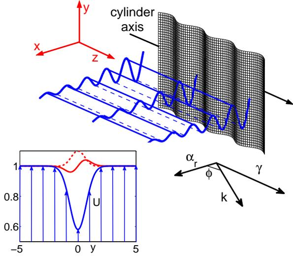
Figure 1: Perturbation geometry scheme, mean flow  $U$  in the wake at  $Re = 40$  and  $x_0 = 10$  (blue curve), symmetric and asymmetric initial conditions in terms of  $\hat{v}(t = 0, y)$  (red curves).
