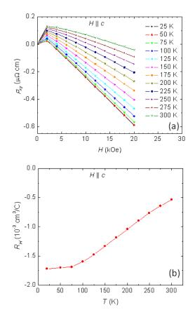
**Figure 2.** (a) The Hall resistivity  $\rho_{xy}$  at several temperatures as a function of magnetic field. (b) The plot of the Hall coefficient  $R_H$  with temperature obtained from (a).
