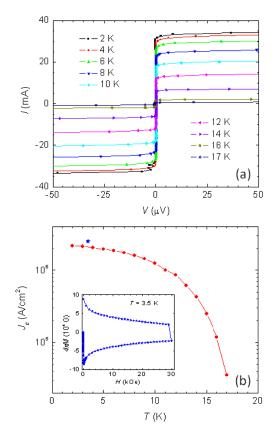
**Figure 3.** (a) The zero-field current-voltage characteristics in Co-doped BaFe<sub>2</sub>As<sub>2</sub> thin film at T = 2, 4, 6, 8, 10, 12, 14, 16, and 17 K. (b) The critical current density  $J_c$  at different T obtained from (a). The data point at 3.5 K (star) is obtained from the magnetization hysteresis loop shown in the inset.
