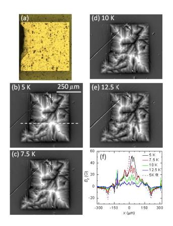
**Figure 4.** (a) Optical image of the film used for magneto-optical imaging. The differential magneto-optical images of the remanent state in Co-doped  $BaFe_2As_2$  thin film at (b) 5 K, (c) 7.5 K, (d) 10 K, and (e) 12.5 K. (f) The local magnetic induction profiles at different *T* taken along the dashed line illustrated in (b). The dashed line in (f) is a fit to the profile at 5 K using the critical state model.
