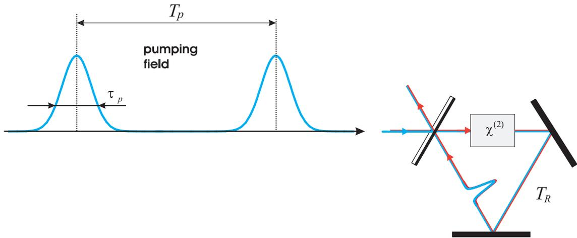
Figure 1: Synchronously pumped OPO
