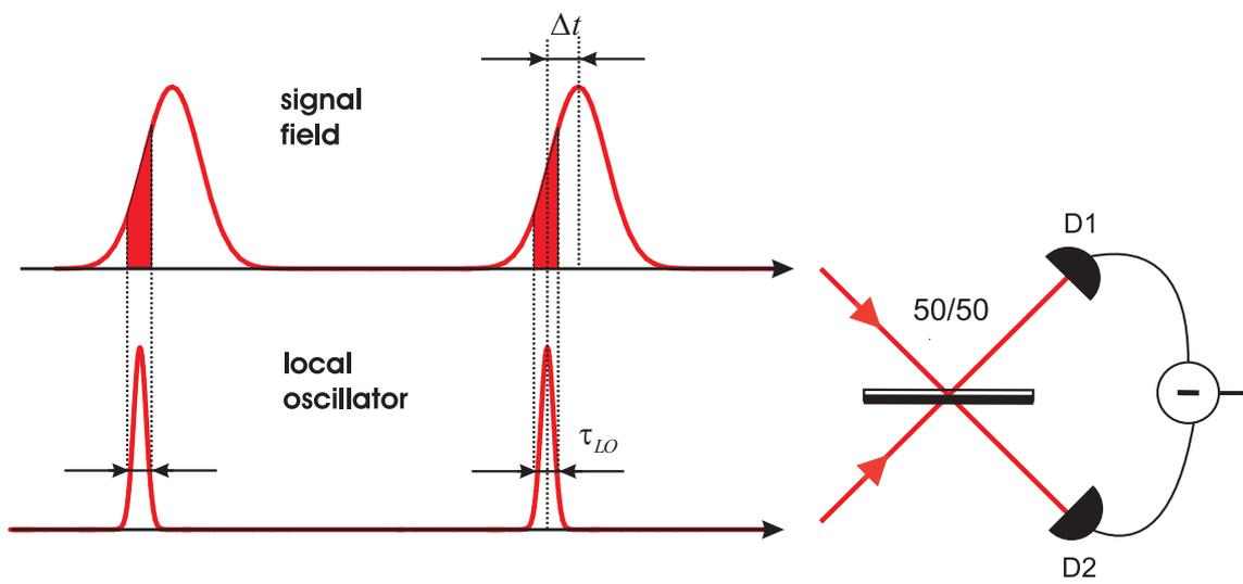
Figure 2: Balanced homodyne detection
