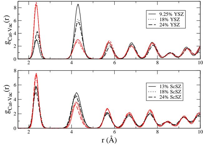
Figure 4: Cation-vacancy radial distribution functions for YSZ (top) and ScSZ (bottom) for different dopant concentrations at 1250 K. The red curves are the Zr-Vac rdfs while the black curves represent the dopant cation-vacancy rdfs.
