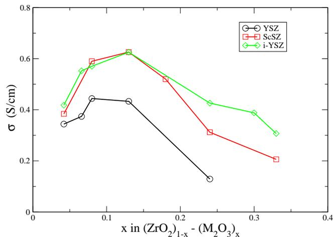
Figure 6: Conductivity versus vacancy concentration for  $i\text{-YSZ}_x$ , YSZ and ScSZ at 1670 K. The data for  $i\text{-YSZ}_x$  has been rescaled by a factor of 0.8 to facilitate the comparison. That  $i\text{-YSZ}_x$  has a slightly higher conductivity, at each  $x$ , than ScSZ is probably a consequence of the potential which has, on average, a less repulsive short-range interactions (see the discussion in reference<sup>25</sup>).
