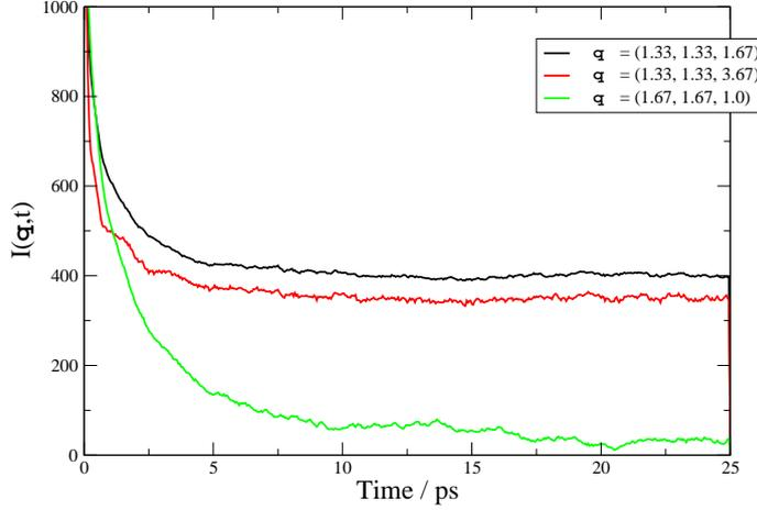
Figure 3: Time scan at constant  $\mathbf{q}$  through the quasielastic diffuse scattering from 13 % YSZ at 1800 K.
