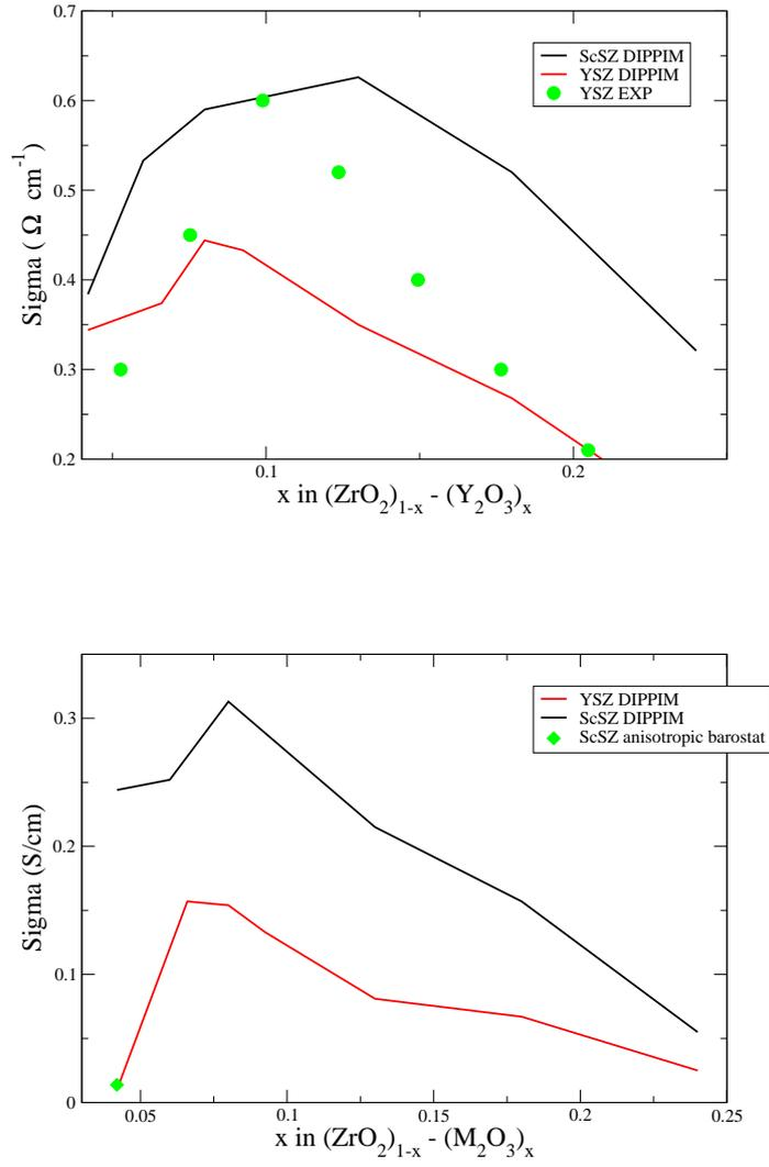
Figure 1: *Top*: MD conductivities vs doping ( $x$ ) for YSZ (red curve) and ScSZ (black curve) at 1670 K. We also report the experimental data from<sup>33,34</sup> for YSZ at the same temperature. *Bottom*: MD conductivities vs doping ( $x$ ) for YSZ (red curve) and ScSZ (black curve) at 1250 K.
