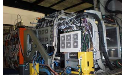
Figure 4.(left) Schematic view of beamline setup. (right) Detector side view showing ScECAL+AHCAL+TCMT
