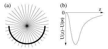
FIG. 3: Argument that a thin metallic hemisphere repels a point charge. (a) At z = 0, the vacuum electric field lines of the point charge are already perpendicular to the hemisphere (side view), so the electric field is unaffected by the presence of the hemisphere. (b) Schematic charge-hemisphere interaction energy  $U(z) - U(\infty)$ : zero at z = 0 and at  $z \to \infty$ , and attractive for  $z \gg R$ , so there must be repulsion for small positive z.
