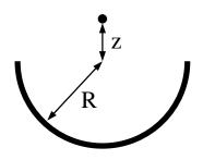
FIG. 2: Example of a geometry in which a neutral metallic object repels a point charge: a point charge centered above a thin metallic hemisphere (side view).
