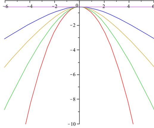
Figure 3: Plot of a Case 4 trajectories. The lowest (innermost) red curve is the parabola of free fall corresponding to  $\lambda = 0$ . Above that one the curves correspond to  $\lambda = N/mg = 1/4$  (green),  $\lambda = 1/2$  (brown),  $\lambda = 3/4$  (blue) and finally the horizontal straight line (violet) corresponds to  $\lambda \rightarrow 1$ .
